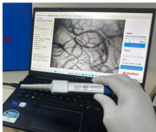
Fig. 1 - CytoCam-IDF handheld video microscope used for visualization of microcirculatory parameters in our department, based on IDF technology. The CytoCam is a pen-like device and is held as such. The low weight of the device (120 g) minimizes pressure artifact problems that were present in the earlier heavy devices. The camera is connected to a device controller based on a medical grade computer or a suitable portable device such as laptop or tablet, which is used for image storage (from https://braedius-medical.com/products/ ). IDF=incident dark field.
